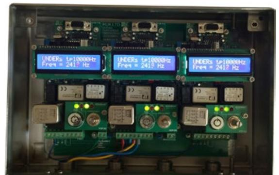
The VOP 03 set point is not influenced by temperature and friction like older mechanical devices. It will provide a very repeatable trip set point for long periods with no adjustments giving trouble free reliable overspeed protection.
